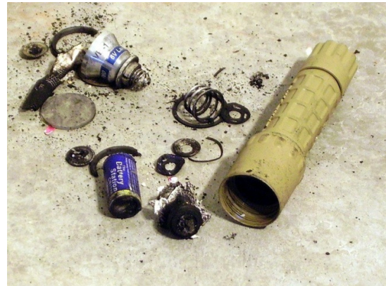
Pic 2 – exploded lithium batteries
