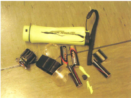
Pic 1 – gassing alkaline batteries
